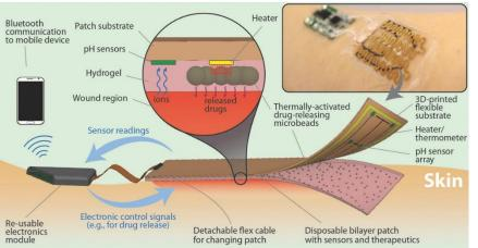
monitor multiple features, building the sort of picture required to fully understand the wound status. In the past, the exudates have limited the biosensors' sensitivity. In the new design, the researchers enclosed the sensors in a porous membrane, protecting their parts and increasing their operational stability.
